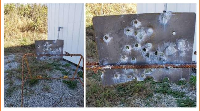
As can be seen in the photo, there appear to have been several impacts to the crossbar. Not only does this lesson the life of the target stand, it is dangerous. Furthermore, non-bullet rated steel should not be shot at the range. As written in the range rules:
